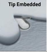
Inserted tooth design will greatly increases the body-to-tip braze area for greater support and tip strength.
