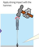
the loosening direction and it loosens even the stripped screw.
