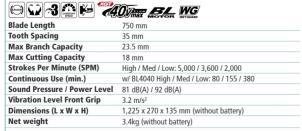
Standard Equipment: Blade Cover, Chip Receiver
