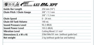
Standard Equipment: 25cm Guide Bar and Chain with 1.1mm Gauge / 3/8" Pitch / 90PX CC
