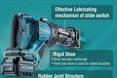
The tool body is separated nto the upper and lower housings which joined with vibration absorbing cushion rubbers to reduce load on battery and terminal
