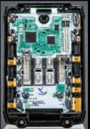
Terminal short-circuit prevention structure. The protection wall is provided between terminals against water and dust.
