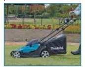
Deck cover is added to under Deck (the contact surface with grass) to reduce the force required to push the machine
